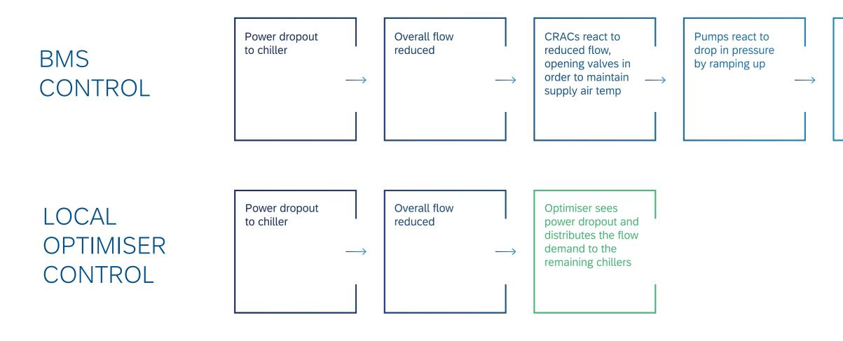
System will take time to find new equilibrium – period of "hunting"  $\longrightarrow$ which could lead to temperature instability in DC Redundancy not maintained and additional equipment issues could lead to SLA breaches
