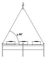
Lift via 4 slings (provided by others) attached to the lifting holes provided to the 4 corner legs as indicated
