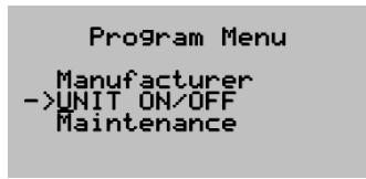
To turn the unit on press the key to enter the program menu. Using the and keys select the Unit On/Off option and press :
