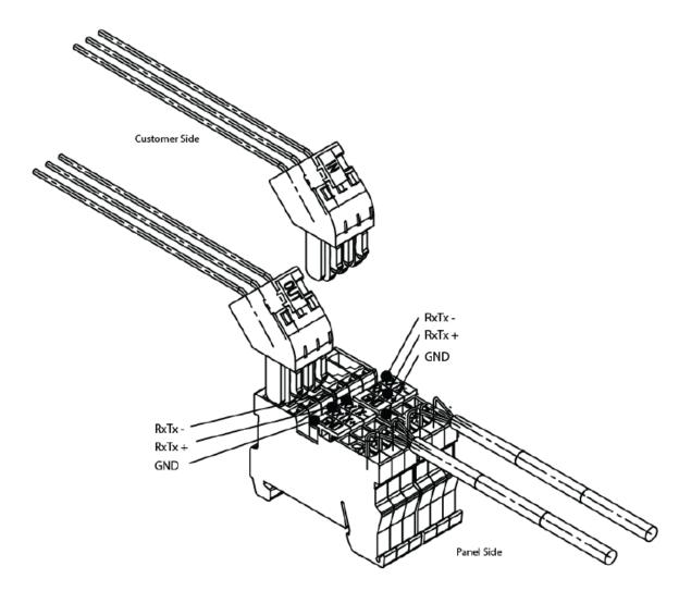
IMPORTANT: The plugged termination ensures that the connections are made simultaneously. Failure to attach the cables in this way may cause damage to the controller.
