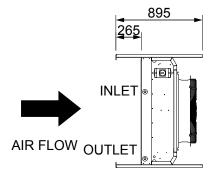
Inlet (Top) = Discharge Line Outlet (Bottom) = Liquid Line
