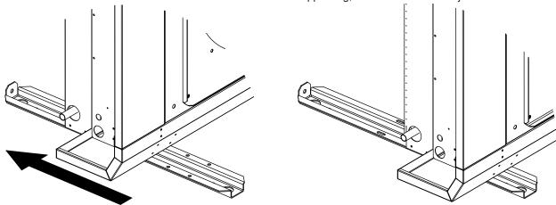
Step 4. Lower and rest the unit down to floor and reposition and secure the upper legs as described in Step 3. Step 5. In line with vertical discharge lifting instructions lift the unit slowly into vertical orientation. Care should be taken to ensure the unit does not drop into position and that damage is not sustained prior to lifting the unit into final position. Step 6. The unit may be lifted into its final position.
