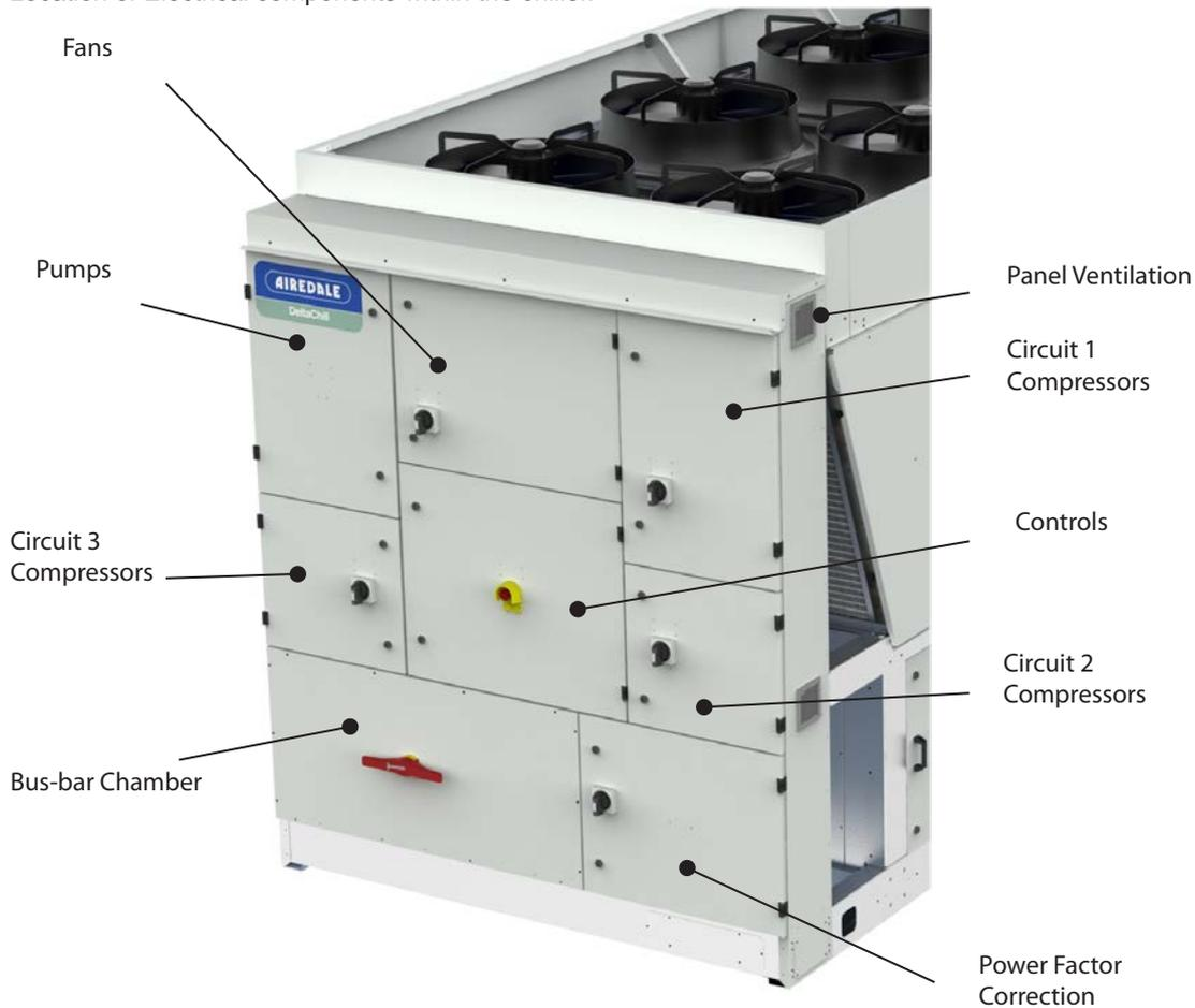
A weatherproof electrical power and controls panel shall be situated at the end of the unit and contains:
