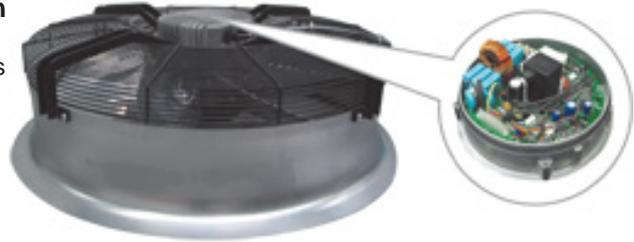
The long bell mouth design provides improved aerodynamics, up to 10% more air movement, and an extended vertical throw of air to reduce the chance of air re-circulation. As standard the enclosure is complete with an integral finger proof grille.
