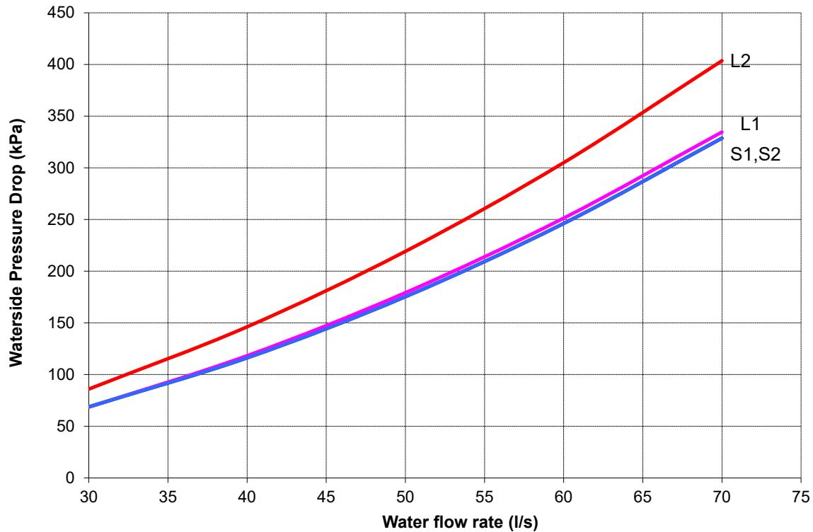
**Performance Data****Waterside Pressure Drop (Unit) (kPa) 2 Row Coil****18 Fan****CAUTION ▲**
