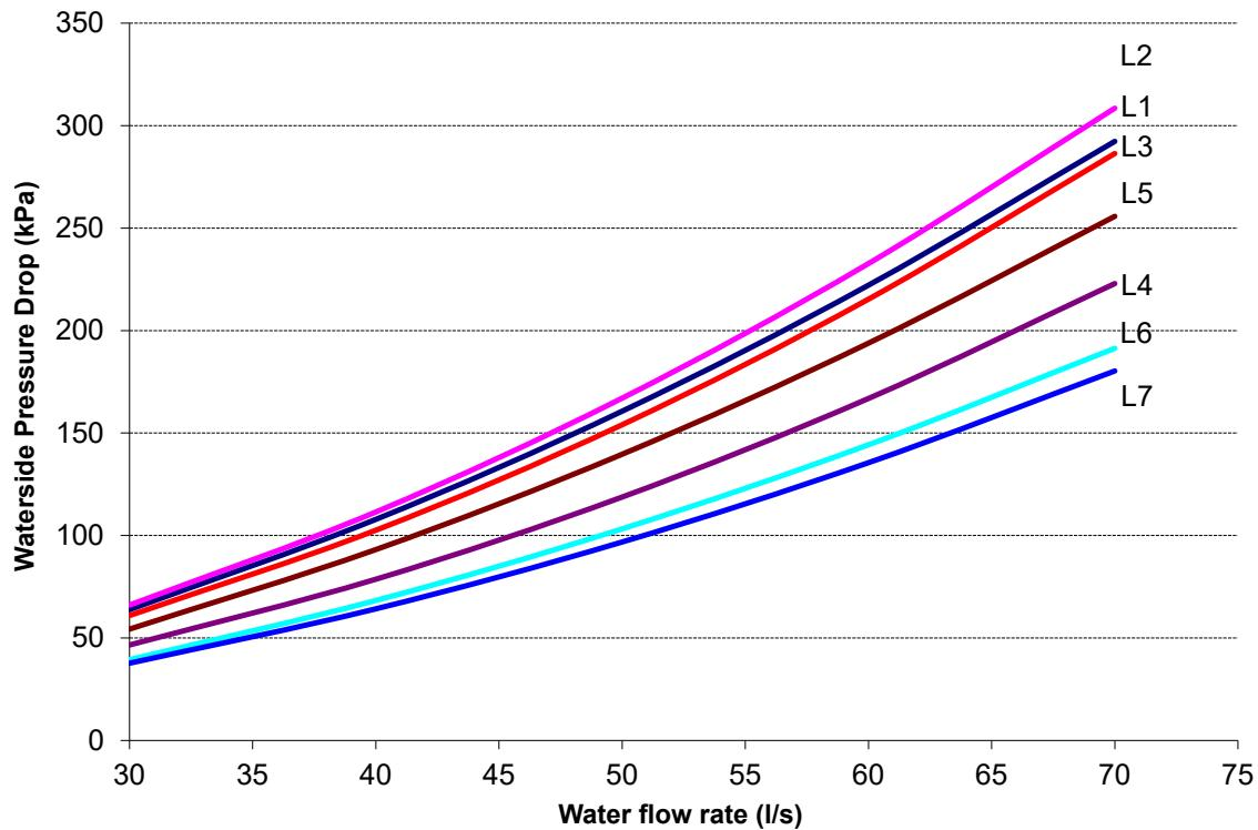
(1) Chiller pressure drop refers to standard unit only. For optional extras and pipework, please contact Airedale.
