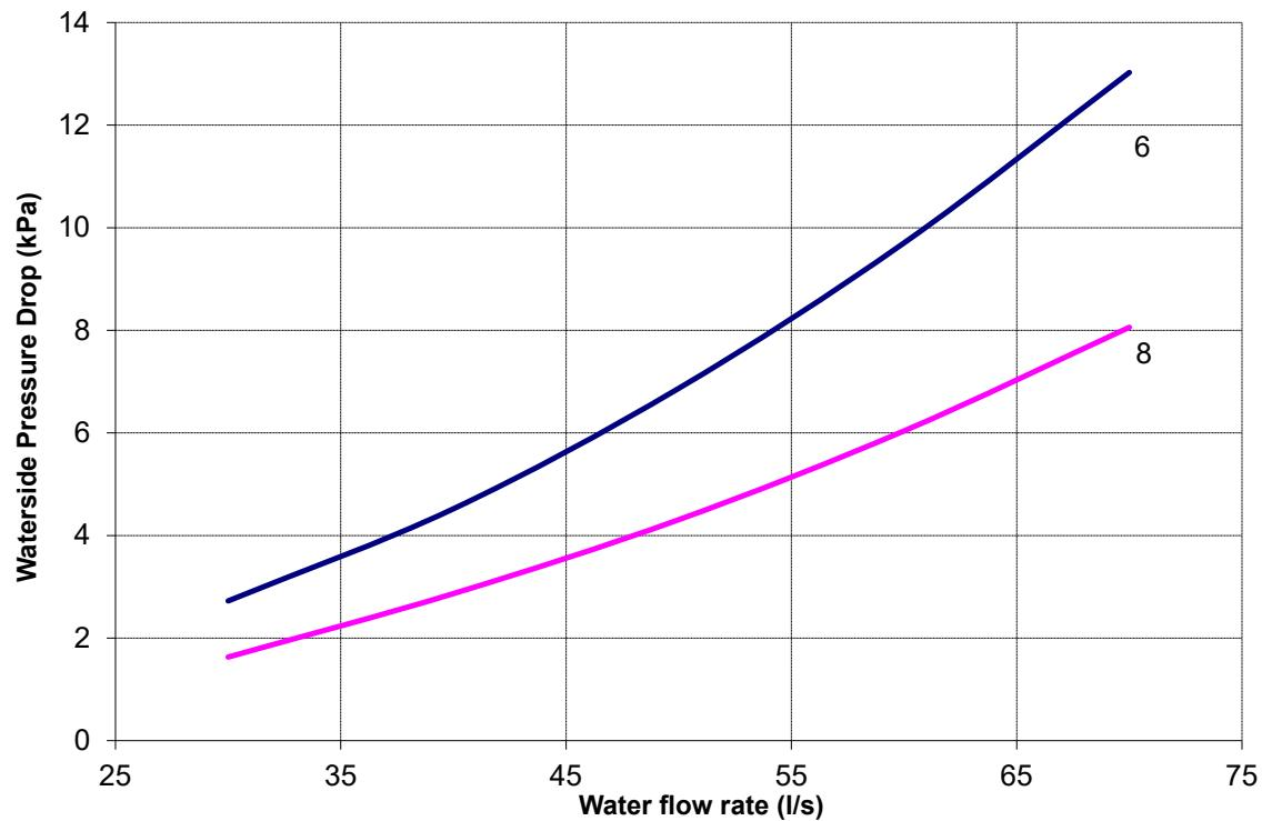
The above curves relate to the strainer size (inches). Data based upon the strainer being clean.
