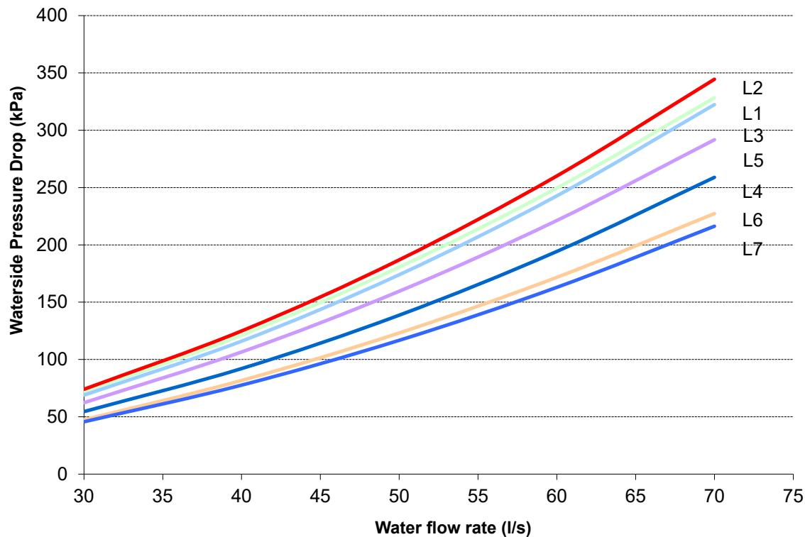
**Performance Data****Waterside Pressure Drop (Unit) (kPa) 2 Row Coil****20 Fan****CAUTION ▲**
