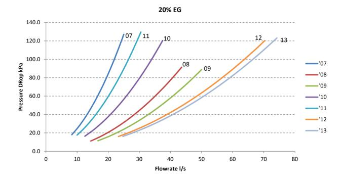
Hydronic Data Evaporator Pressure Drop - 20% Ethylene Glycol
