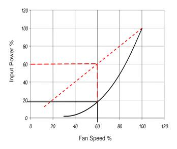
Fan speed of 60% Voltage regulated input power required 60% EC input power required 18%
