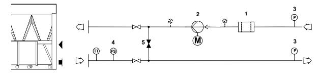
**CAUTION** A The correct operation of the flow proving device is critical if the chiller warranty is to be valid.
