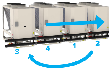
Figure 3: rotation operation logic.
