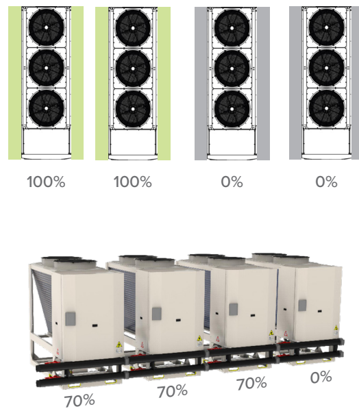
Figure 11: different operation behaviour at part load (50% of installed capacity) for a non-inverter modular system (left) and Full DC inverter system (right)
