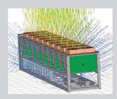
CFD analysis was used to determine the optimum fan and heat exchanger size and the best distribution and total airflow through the V - block to minimise power consumption
