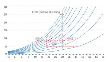
y axis: Moisture Content (g Water / kg Dry Air) x axis: Dry Bulb Temperature (°C)
